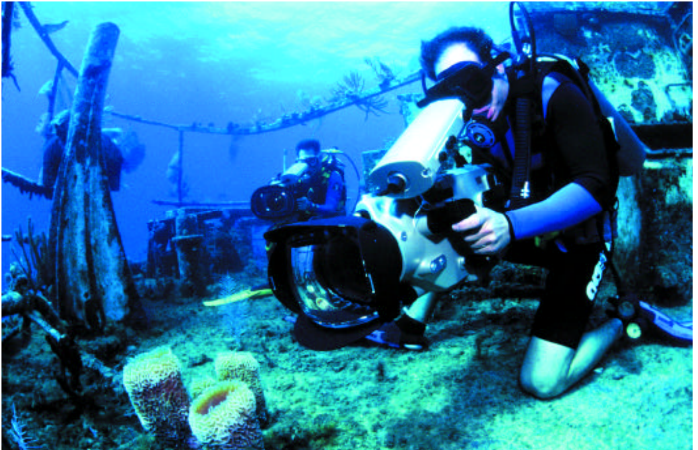
Sony HDW-700 high definition cameras fit snugly into the Amphibicam housings, which allowed ASL to move quickly from underwater to topside shooting in only 5 minutes.
